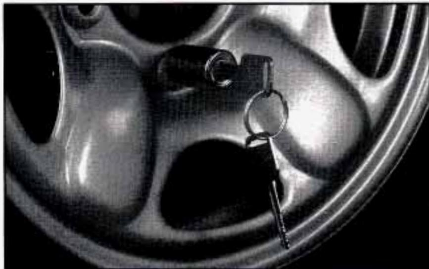
Insert your key into the wheel lock on the spare tire and pull the wheel lock off.
