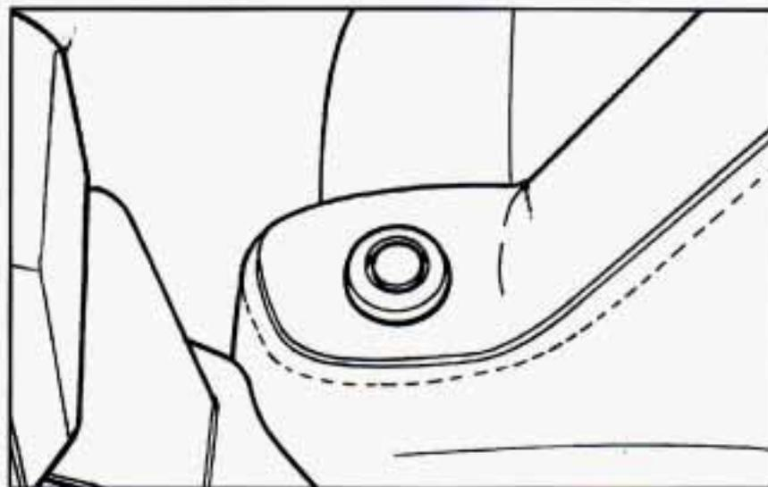
2. Pull the knobs on both sides of the seatback. If you have the split rear seat, you can fold half of the seat by pulling only the knob on the side you wish to fold.
