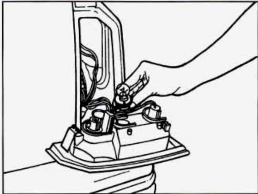
3. Disconnect the bulb from its socket by twisting and then pulling the bulb out.
