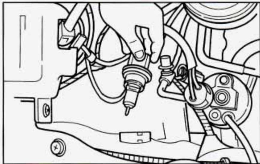
4. Pull the lock ring and the headlamp bulb straight out. Save the lock ring, and use it with the new bulb.
