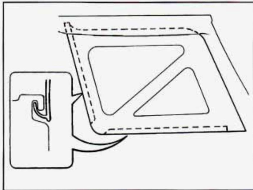
After completing installation, make sure that the front and bottom ends are securely hooked and the rear top end of the window is under the canvas top.
