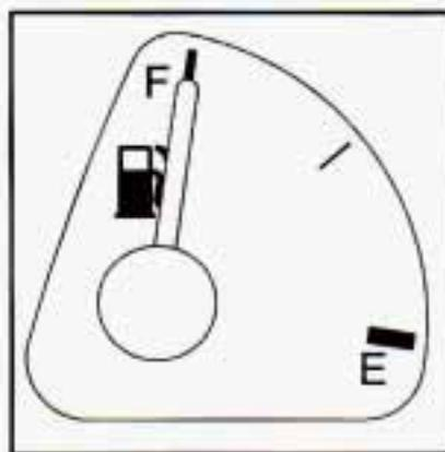
Your fuel gage shows about how much fuel is in your tank. When the gage first indicates E (EMPTY), you still have about one or two gallons (4 to 8 L) of fuel left in your tank, but you need to get more right away.
