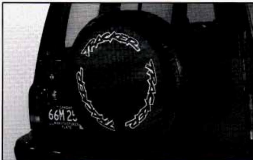
The spare tire is mounted on your tailgate. Pull the cover off of the spare tire.
