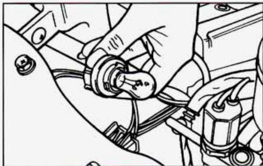
3. Push the bulb in, turn it to the left and pull it out.
