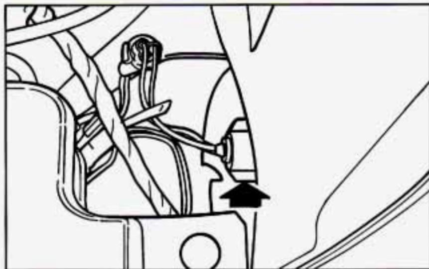
To replace the parking and turn signal bulb:
