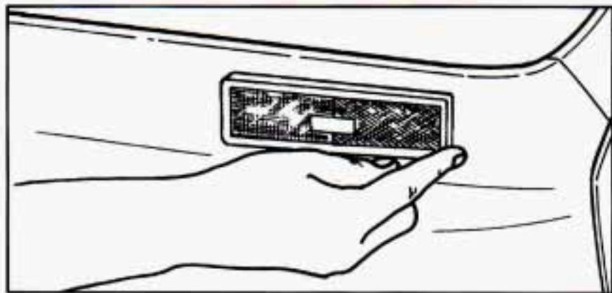
1. Push the sidemarker housing toward the back of the vehicle to release the clip and pull out the front edge. The housing should pull away from the vehicle.
