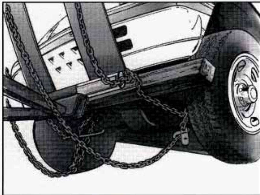
Position a 4" x 4" wood beam across the sling chains and against the lower control arm front attachment brackets. Position the lower sling crossbar in front and against the 4" x 4" wood beam.
