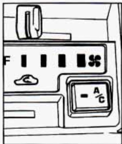
The air conditioning system uses the same controls as described previously. The function of each lever is explained under “Climate Control System” in this part. The incoming air is cooled and dehumidified instead of being heated.
