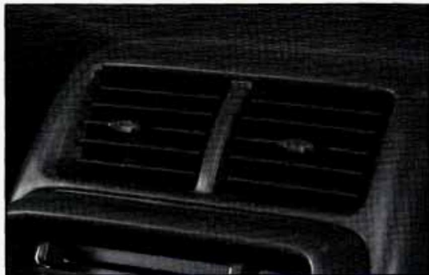
Your vehicle has air outlets that allow you to adjust the direction and amount of airflow inside the vehicle. Move the louvers up or down to direct airflow to your preference. Increase or reduce the amount of airflow by opening and closing the louvers.
