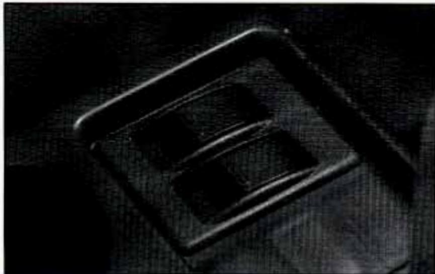
The driver-controlled switches for the rear windows are located on the center console.
