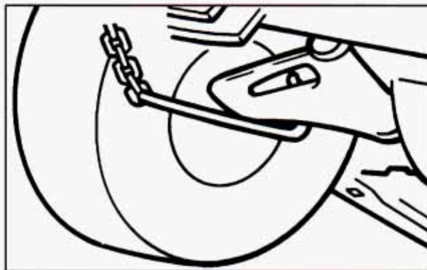
Attach J-hook chains on both sides to the rear of lower control arms inboard of the spring.
