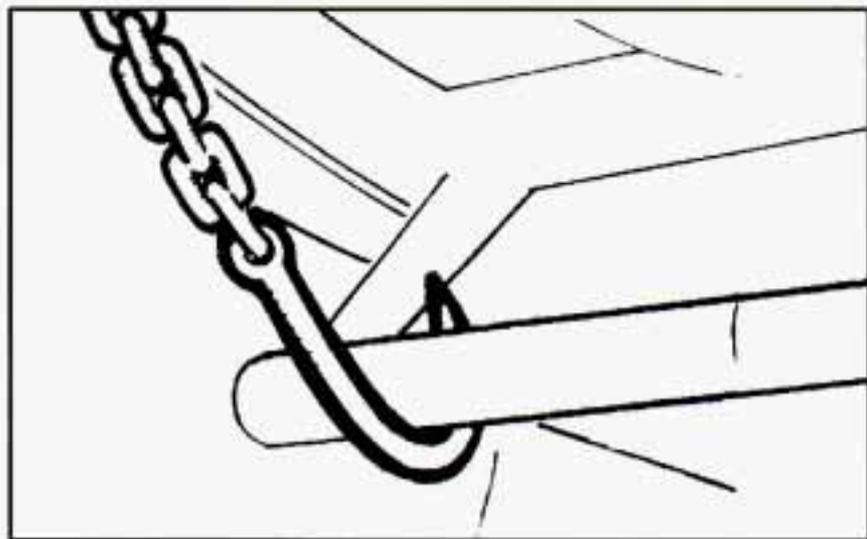
Attach J-hooks around the axle tube.
