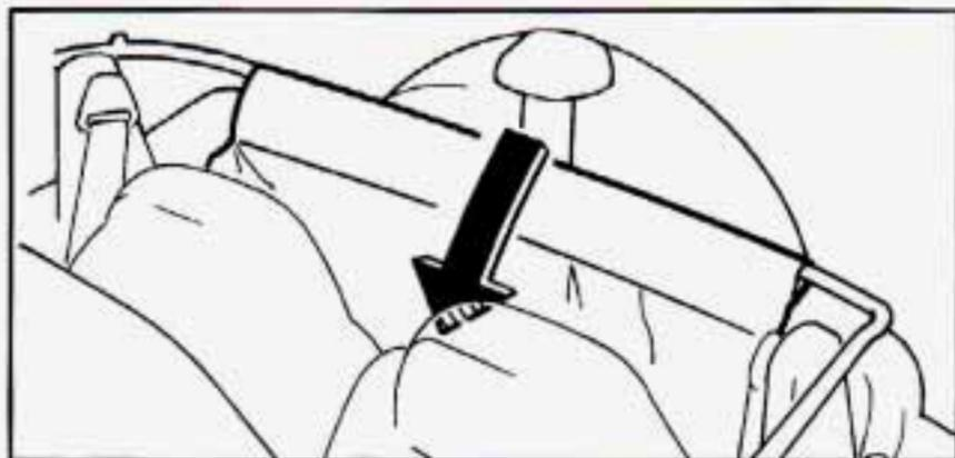
13. Lower the folded canvas behind the rear seatback(s). Make sure that the rear seat belts around the shoulder anchor are clear from the folded top.
