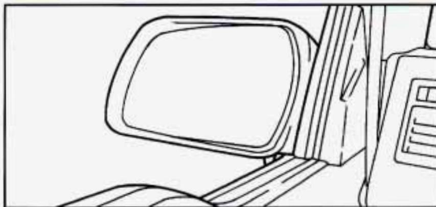
Adjust these mirrors by hand so that you can just see the side of your vehicle when you are sitting in a comfortable driving position.
