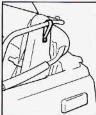
14. Fasten the upper top bow with the belt on the driver's side seat belt shoulder anchor bracket.
