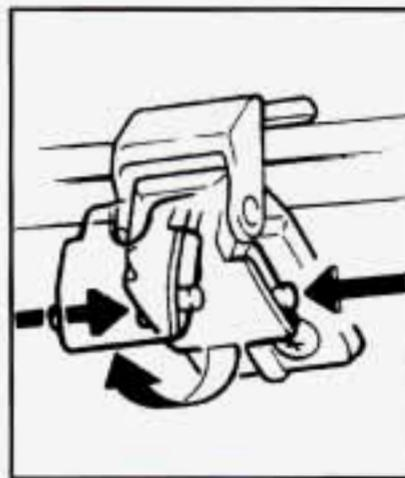
5. Lower the sun visors and push both sides of the lock buttons on the front latches.
