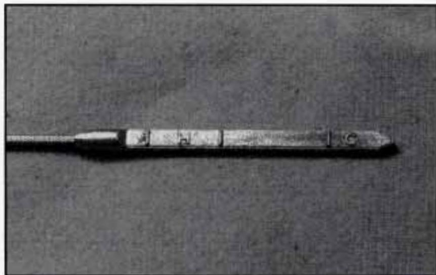
3. Check both sides of the dipstick, and read the lower level. The fluid level must be in the COLD area for a cold check or in the HOT area or cross-hatched area for a hot check.
