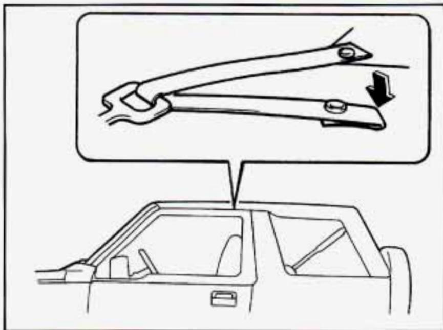
3. Unfasten the snaps on the driver's and passenger's sides of the roof side tension belts, located above the doors on the outside of the vehicle, underneath the canvas top.
