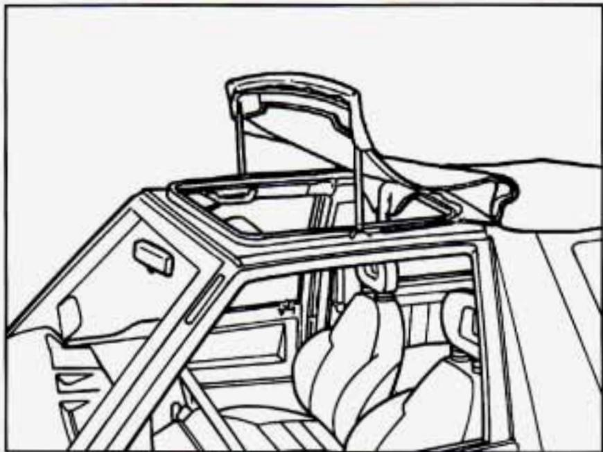
4. Swing the front top bow up and back while folding the canvas top out from between the top bow and the roof support. Be sure that you don't pinch the canvas top between the front top bow arms and the roof rails.
