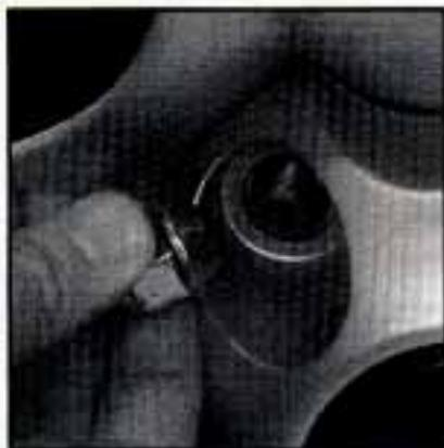
7. Replace the wheel nuts with the rounded end of the nuts toward the wheel. Tighten each nut by hand until the wheel is held against the hub.
