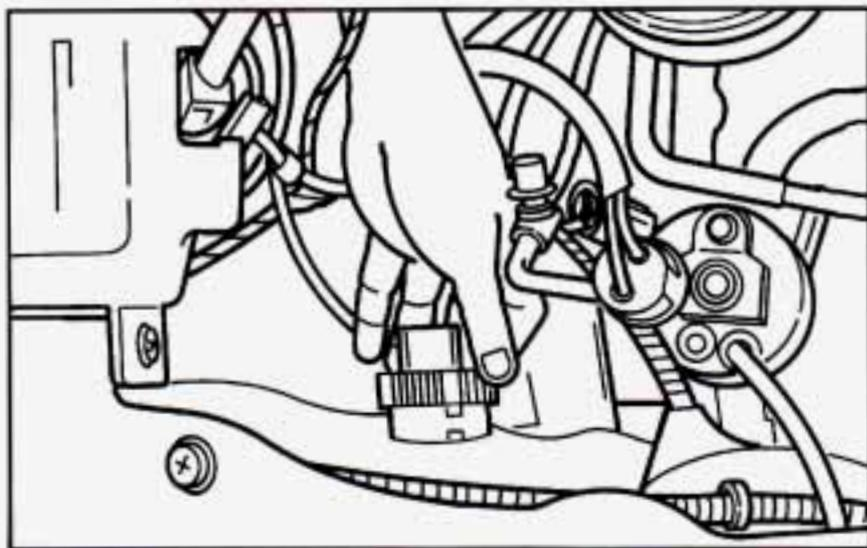
3. Turn the lock ring to the left to release the bulb.
