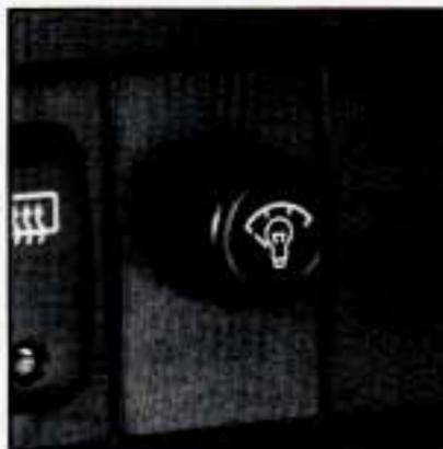
This knob controls the brightness of your instrument panel lights. Turn the knob to the right to brighten the lights or to the left to dim them.
