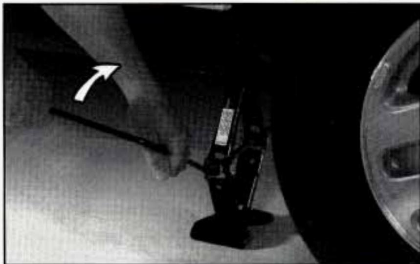
3. Raise the vehicle by turning the jack handle to the right. Raise the vehicle far enough off the ground so there is enough room for the spare tire to fit.
