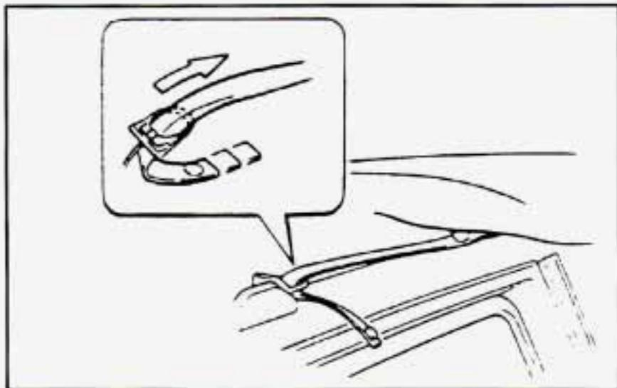
9. Pull the tension belts located above the door frame out through their rings.
