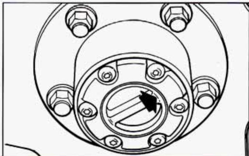
Your vehicle may have either manual or automatic freewheeling hubs. You must lock the hubs before you use **FOUR-WHEEL HIGH (4H)** or **FOUR-WHEEL LOW (4L)**.
