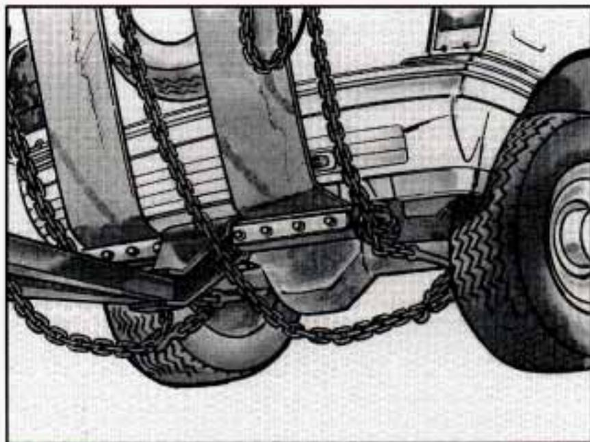
Position the sling crossbar under and forward of the rear bumper.
