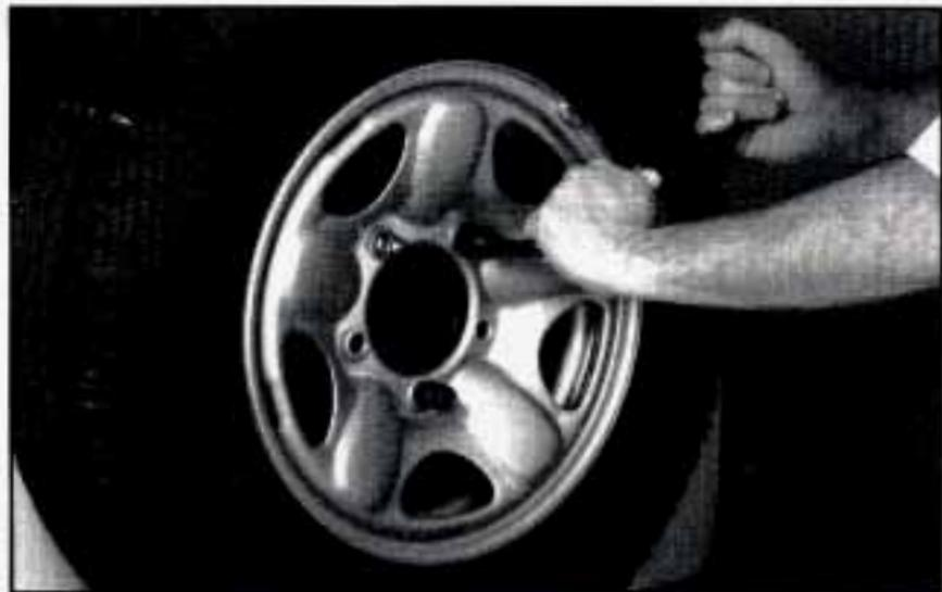
Remove wheel nuts with the wheel wrench.
