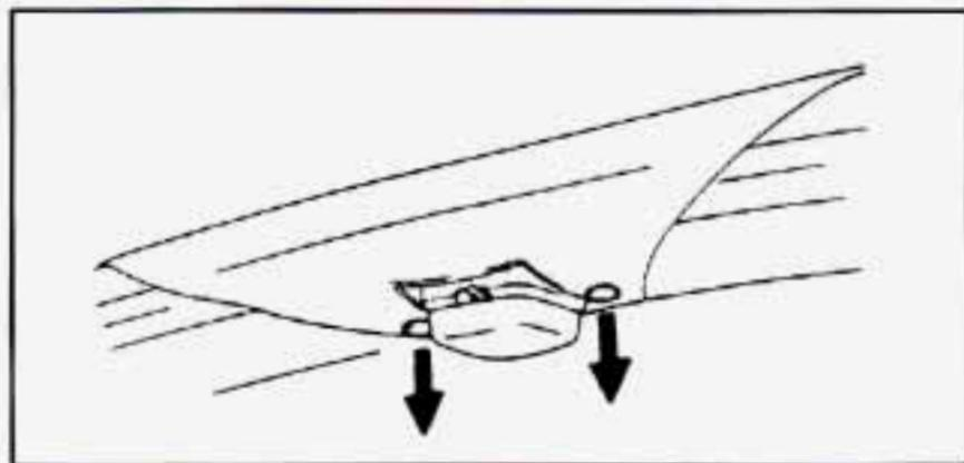
4. Unfasten the snaps that secure the canvas top to the roof piece. The snaps are located on either side of the dome lamp.
