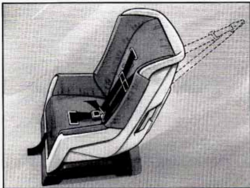
If your child restraint has a top strap, it should be anchored. If you have a two-door model, don't use a restraint like that in your vehicle because the top strap anchor cannot be installed properly. You shouldn't use this type of restraint without anchoring the top strap.
