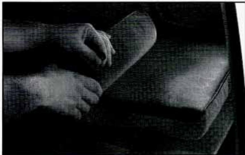
2. While pulling up on the lock knob, fold each rear seatback down. Both rear seatbacks must be folded down in order to move the seat forward.
