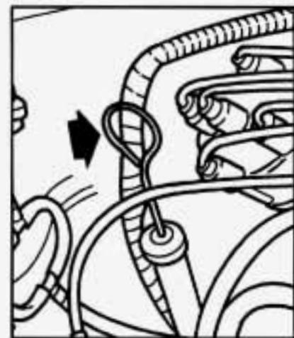
1. The automatic transmission dipstick is a black ring handle located in the rear of the engine compartment toward the passenger's side of the vehicle. Pull out the dipstick and wipe it with a clean rag or paper towel.
