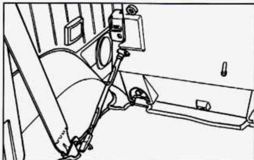
8. Attach the support bar to the floor bracket.
