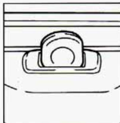
To lock the door from the inside, push down the button on the door. To unlock it, pull up on the button.
