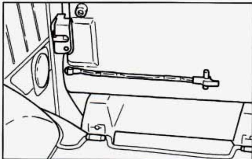
6. Find the support bar on the bottom of the seat. This bar keeps the rear seat from unfolding.
