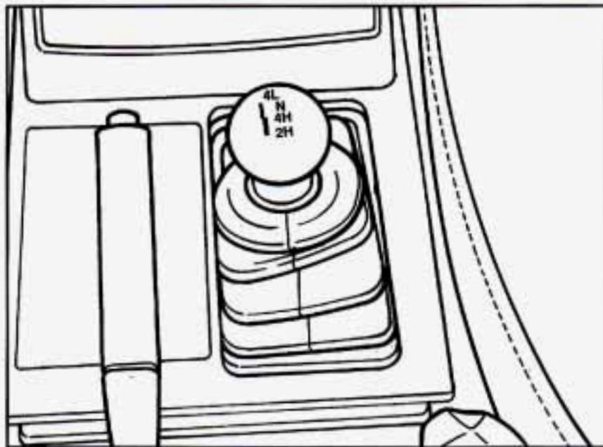
The transfer case shift lever is on the floor to the right of the driver. Use this lever to shift into and out of four-wheel drive. An indicator light comes on when the transfer case is in **FOUR-WHEEL HIGH (4H)** or **FOUR-WHEEL LOW (4L)**.
