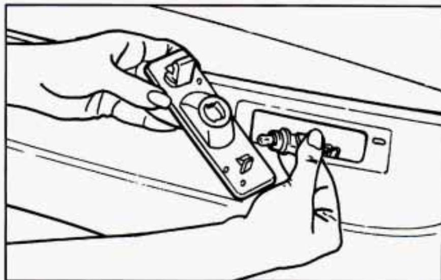
2. Turn the socket to the left and pull it out of the housing.
