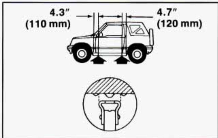
2. Position the jack and raise the jack lift head until it fits firmly onto the notches nearest to the flat tire. (Under the vehicle near each wheel, there are notches in the vehicle's rocker flange.)
