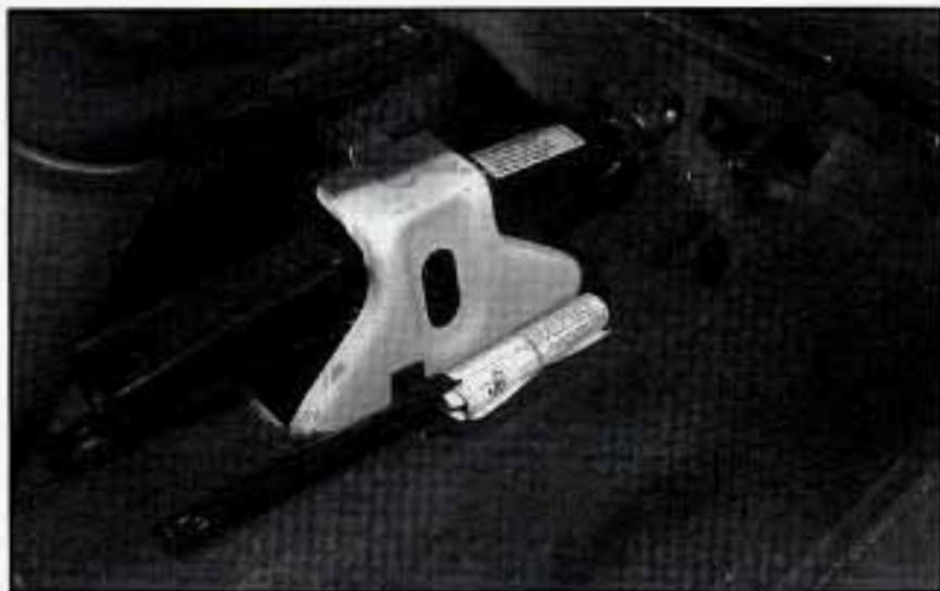
The jack and wheel wrench are under the front passenger's seat.
