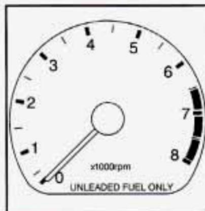
The tachometer shows engine speed in thousands of revolutions per minute (rpm). You can use it while driving to select correct shift points. The tachometer may not return to zero when the engine is not running.
